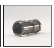
The VibRotor is a vibrator rotor intended for use in small pipes. It excels at being efficient even at low pressure. The VibRotor is equipped with 2 tangential 85° sprays and 2 tangential 45° sprays angled towards the pipe wall, as well as 12 blades running along its length.
