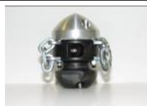
#3 - Alu-protection-head with link-chain-rotor.
