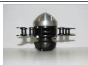
#6 - Alu-protection-head with bicycle-chain-rotor.
