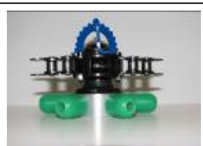
#11 - Central cutter with bicycle-chain-rotor and guide ring + extensions.
