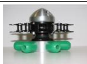
#10 - Alu-protection-head with bicycle-chain-rotor and guide ring + extensions.
